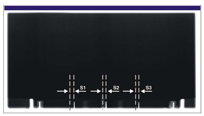
2. After taking the exposure, measure the distances \$1, \$2 and \$3 with the SIDEXIS XG measuring ruler.
