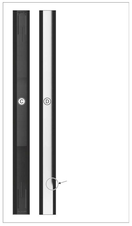
On the exposure with coarse adjustment (**D**), the exposed area is just barely visible at the right margin of the image field. Even in this extreme case, an adjustment would still be possible.
