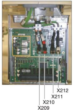
12. Plug the cables into the sockets of board DX88 according to their color coding:
